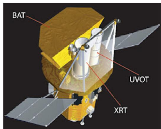
Swift's three telescopes work together to learn as much as possible about gamma-ray bursts: X-ray (XRT), ultraviolet and optical (UVOT) and burst alert (BAT). Credit: NASA
